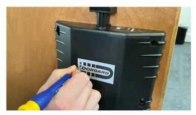
The programming button is at the front of the Dorgard and can be accessed by inserting a small screwdriver or equivalent into the hole - as shown in the image to the left.
